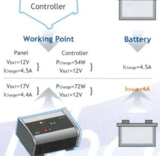
The comparison between MPPT and traditional controller shows that the energy output of the panel is up to 30% higher with the use of MPPT. This leads to an average increase of about 15%.
